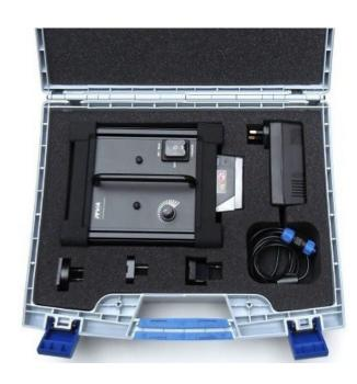
The Field-Flow Compact is a battery powered peristaltic pump designed for low flow ground water sampling in inaccessible areas. The highly portable unit can be an advantage where mains power or a vehicle (battery) are unavailable.
