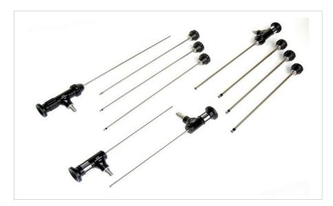
A wide range of set viewing direction, adjustable focus rigid borescopes. High quality rod lenses are used, surrounded by glass fibres for bright and even illumination of the subject. These instruments are watertight and designed to take pressures of up to 4 bar. Maximum operating temperature 110°C.
